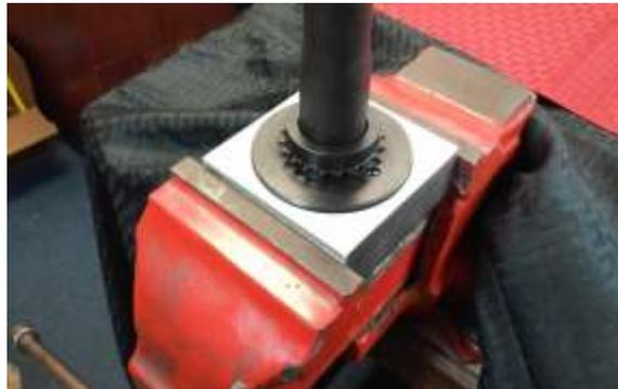
5. Insert the #14 drill bit (non-cutting end) or AR-15 gas tube (gas block end, not receiver end) into the gas tube hole of the Barrel Adapter Assembly to align it Top Dead Center (TDC) with the Installation Fixture and barrel extension pin.
