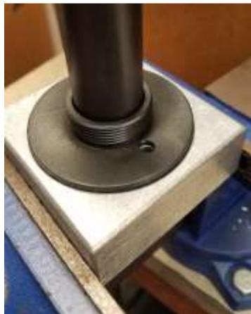
6. Fully seat the Barrel Adapter Assembly into the Installation Fixture. Press down on Barrel Adapter Assembly throughout the installation process to ensure it remains against the face of the Installation Fixture. Check again to confirm that the Barrel Adapter Assembly gas tube clearance hole remains Top Dead Center (TDC).
