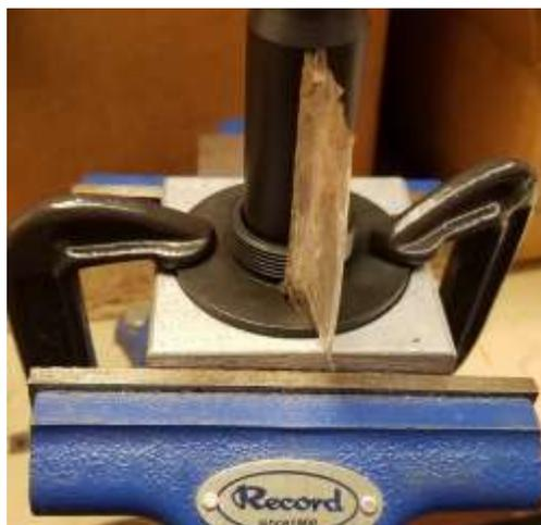
10. Test fit your barrel nut and handguard to ensure it is properly aligned to the barrel. If the alignment is correct, continue to Step 11. If it is not correct, adjust the clamps to bring it into proper alignment. When properly aligned, snug down the clamps.
