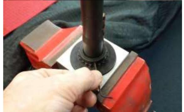
8. Recheck that the drill bit or gas tube slides free and does not bind. Press down on Barrel Adapter Assembly throughout the installation process to ensure it remains against the face of the Installation Fixture.
