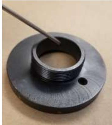
5. Install the barrel adapter onto the stripped barrel. Confirm the dowel pin lugs are to the barrel extension end, and set screws are to the muzzle end of the barrel. Keep the Barrel Adapter Assembly gas tube hole at the Top Dead Center (TDC) location. This is the same position you selected when choosing the slot the barrel extension pin uses. They must be aligned together.
