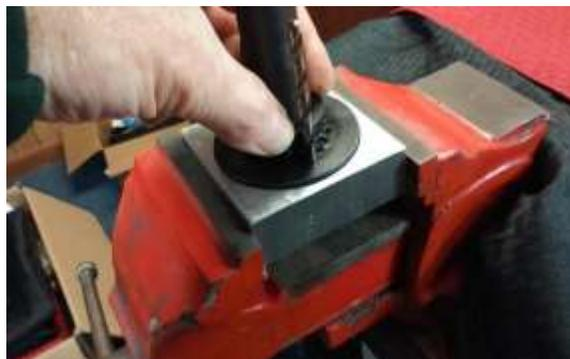
9. Begin alternately tightening the set screws approximately 1/8 turn at a time.
