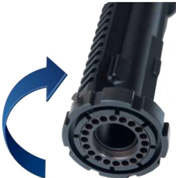
4. Make sure all barrel wrench lugs are fully seated in the Receiver Adapter clearance holes before tightening. Using the AR barrel wrench and calibrated torque wrench, tighten the Receiver Adapter to 30 ft-lb (40.5 N-m). Torque is measured when both wrenches are used together.
