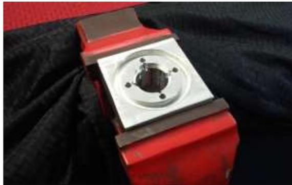
2. Insert the stripped AR barrel into the Installation Fixture. Check that the barrel alignment pin is fully seated in the corresponding Installation Fixture alignment slot. Push the barrel into the Installation Fixture until the barrel is fully seated.
