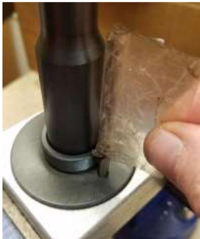
9. Ensure the barrel adapter is flush to the installation fixture and clamp the barrel adapter to the fixture. Leave enough room between the clamps and the barrel adapter to install your barrel nut AND your handguard.
