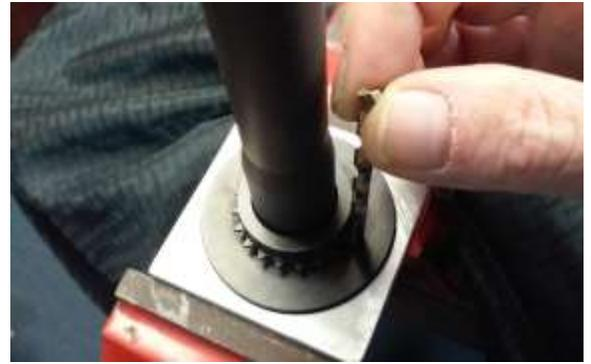
7. Type 1 Only - Using the 1/16" Allen/Hex key loosely between your fingers, lightly take up the distance up to the barrel on all four set screws. Set screws should be done alternately (such as when tightening lug nuts on an automobile). Do not tighten yet. They should just touch the barrel.
