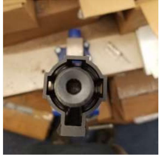
11. Remove handguard and barrel nut from the barrel adapter assembly. Wipe off any excess JB Weld from all exposed surfaces. Any bedding compound that is not removed, will cure and harden. Allow the bedding compound to fully cure for the recommended 24 hours before any more handling.
