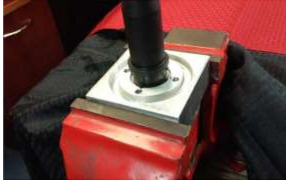
3. Follow the JB Weld manufacturer's recommendations for cleaning the bonding surfaces (inside of Type 3 barrel adapter, and outside diameter of barrel over the chamber). We recommend using acetone or alcohol to ensure bonding surfaces are clean.
