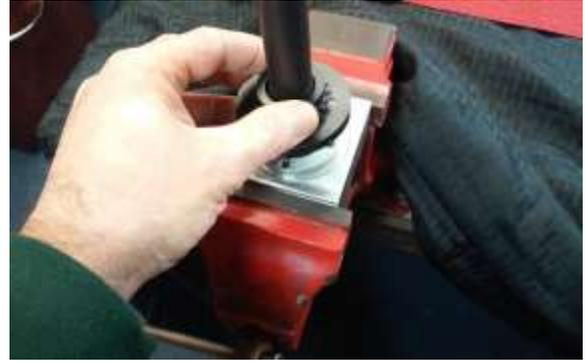
4. Fully seat the Barrel Adapter Assembly into the Installation Fixture. Press down on Barrel Adapter Assembly throughout the installation process to ensure it remains against the face of the Installation Fixture. Check again to confirm that the Barrel Adapter Assembly gas tube clearance hole remains Top Dead Center (TDC).
