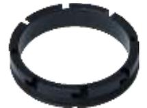
Of importance to note on the Lock Ring, are the FOUR slots milled into the outside of the threaded end. These four slots are provided for the Locking Pin to engage and disengage the Lock Ring. The provision was made so that the Lock Ring can be engaged with a simple quarter turn in either direction. This makes it quick and easy to find a slot for the Locking Pin to use.
